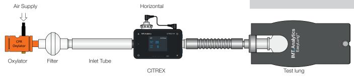
After presetting the CITREX flow analyser and arranging the correct set up, the Oxylator can be started.
