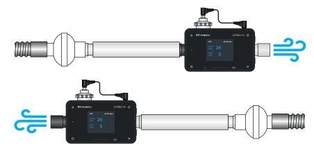
Figure 27: General measurement setup
