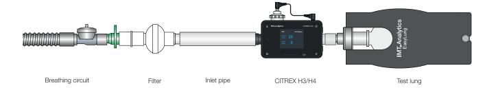
Figure 29: Measurement setup for checking ventilators
