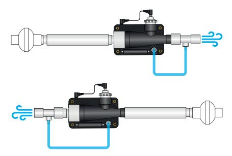
Figure 30: Measurement setup for gases at high pressure
