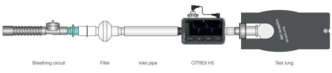
Figure 26: Measurement setup for checking ventilators
