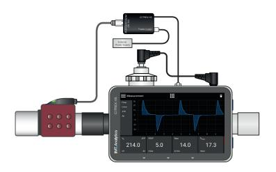
Figure 31: OR sensor connected to the adapter
