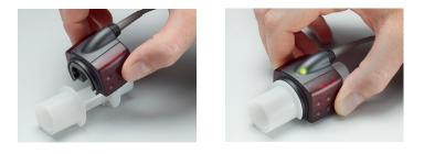
A green LED indicates that the sensor is ready for operation.
