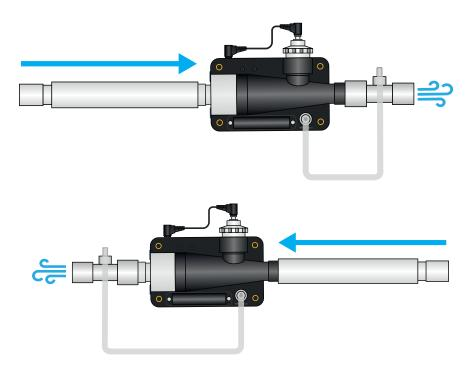
Figure 27: Measurement setup for gases at high pressure
