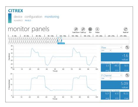
Figure 40: Measurement curves with statistics
