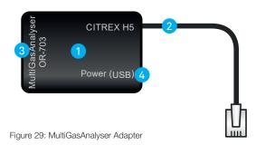
The MultiGasAnalyser Adapter 1 is equipped with a connection cable 2 to the RS232 interface of the CITREX H5, a connection 3 for the OR-703 sensor and a «USB Mini B connector» 4 to supply power to the MultigasAnalyser. This connection on cannot be used as a data interface.
