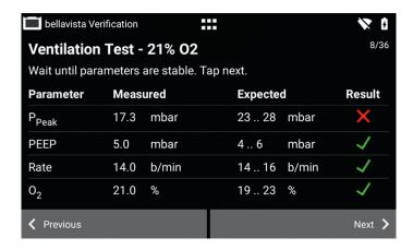
Some tests require a verification of parameters or action on the bellavista screen. In this case, the app displays check boxes which the user checks to confirm the action was performed. Tapping next stores the results for the test report and move to the next screen.
