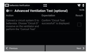
Advanced ventilation test with on/off switch
