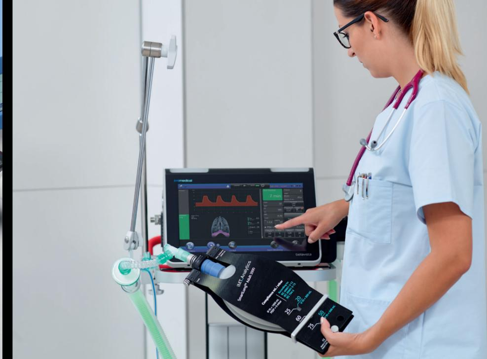
« Test lungs from IMT Analytics simulate a range of realistic ventilation situations during training. »
