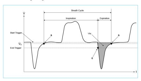
Here, the start trigger should be also placed at S and the end trigger should be placed at E.
