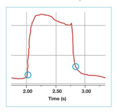
Now here the standard triggers can again be used for the pressure curve: (> 1 mbar) / (< 1 mbar).
