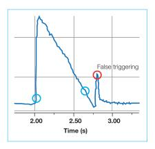
This graph shows the flow curve in the inspiratory channel upstream of the Y-piece. The first two circles indicate the triggers that should be used in this case.
