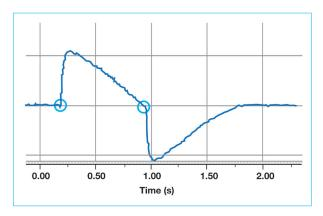
This example shows a flow curve downstream of the Y-piece. The standard triggers (> 3 L/min / < -3 L/min) can be used in this case without any problems.
