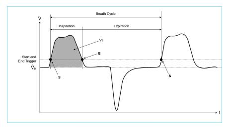
S on this chart represents the start trigger and E represents the end trigger.
